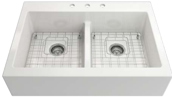
1501-XXX-0127 drop-in recommended Apron-Front Double Bowl *for easy retrofit 34" x 24" x 10" (face= 8") 85.87 lbs min. 36" wide base cabinet required fits standard style base cabinets/apron-front style not required
