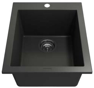
1608-XXX-0126 Dual-Mount Single Bowl 16" x 20" x 8" 22 lbs min. 19" wide base cabinet required; pre-drilled for a single-hole faucet, prescored for easy punch out of additional holes as needed
